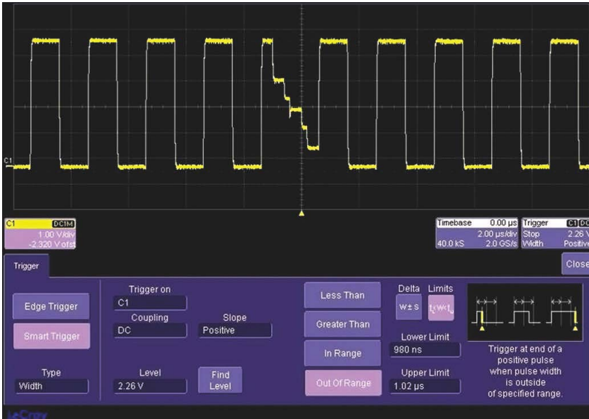
FIGURE 2. By setting a trigger that activates when a waveform characteristic is outside a range, you can ignore acceptable conditions and capture only error conditions, such as the “staircase.”
